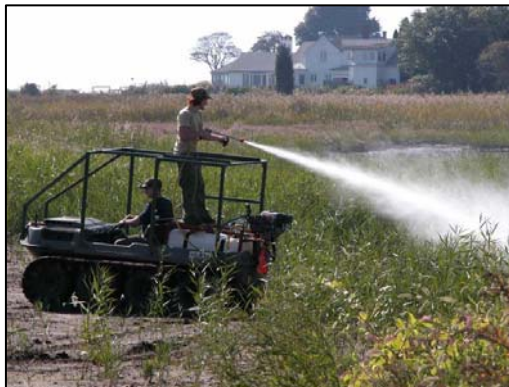
DEP WHAMM Program's Igp ARGO with tower and tank with high-pressure sprayer.
