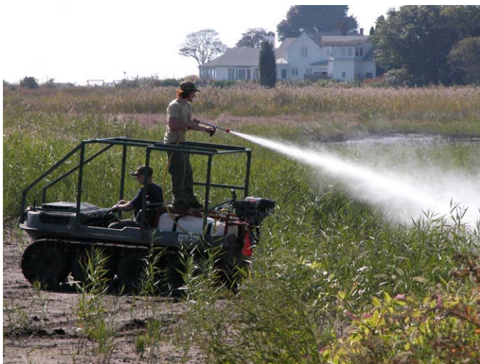
DEP WHAMM Program's Igp ARGO with tower and tank with high-pressure sprayer.
